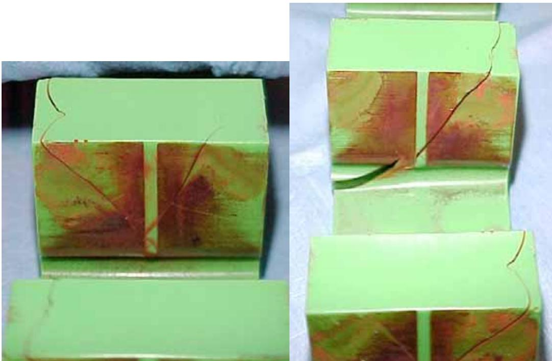
Figure 5 - Flank & Web Cracks on Element Teeth due to Vibratory Loading (Fatigue)
