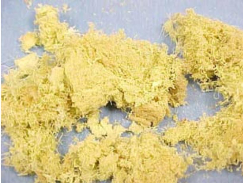
*Figure 6 - Element Wear Debris due to Excessive Angular Misalignment*
