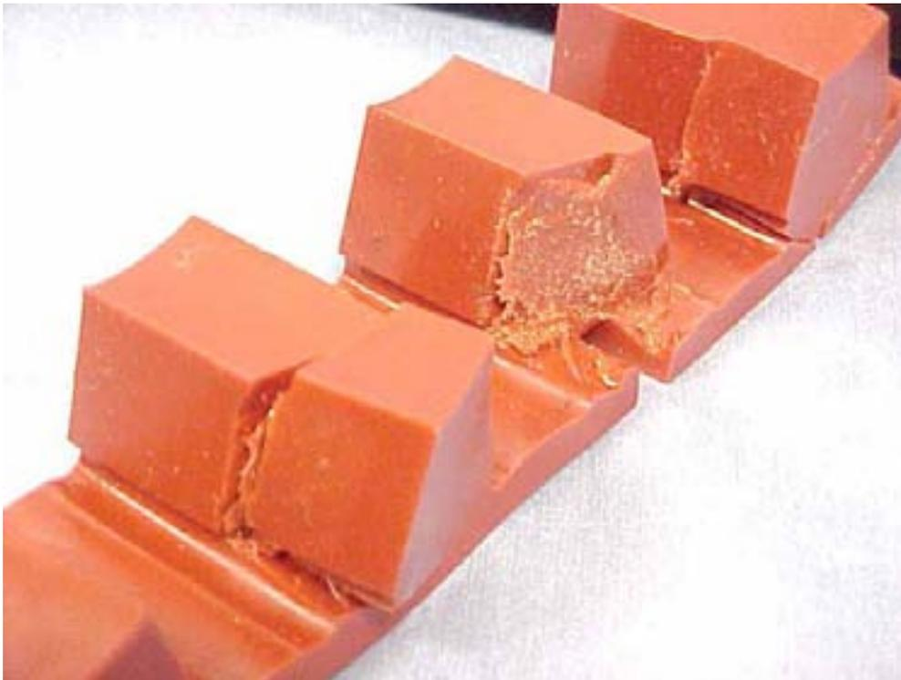
*Figure 3 - Shearing of Element Teeth under Torque Overload*
