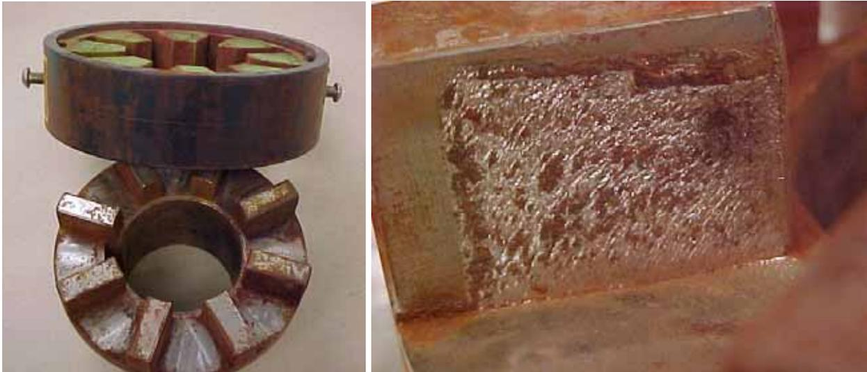
*Figure 9 - Abrasive Wear due to Element Material Fretting Corrosion*
