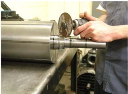
15. (Optional) If there is damage evident to the bearings, they will need to be replaced. Once the rotor is removed, start by cutting off the old bearing inner race on both ends of the rotor. Be sure to line up the cutting wheel with one of the vane slots so as not to damage the rotor or seal sleeve.
