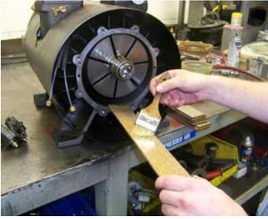
8. Inspect the original vanes for any delamination, chipping or other damage.
