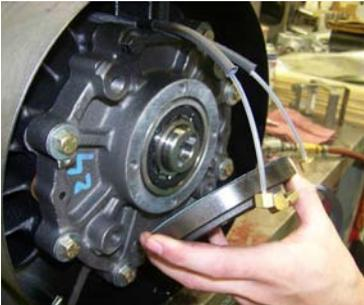
3. Remove the four (4) bolts that hold the rear bearing cover to the rear endplate and note that the wave spring seal is to be re-used.
