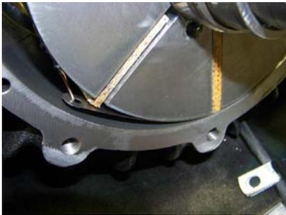
19. Shift the housing so that the intake (Square port) is hanging slightly off of the rebuild work surface.
