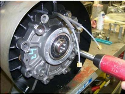
6. Remove the top two end-plate bolts and replace with two (2) 3/8-16 stud/dowels (or de-headed bolts), and then remove the remaining bolts.
