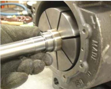
The bearing race shoulder should be tight against the seal sleeve.
