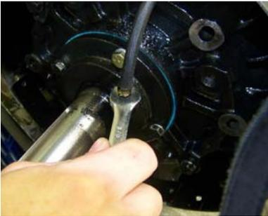
Reconnect the oil lines to the oil pump, and front bearing.
