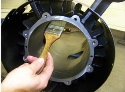
14. Clean the housing of any debris and apply a liberal amount of lubrication to the housing bore.
