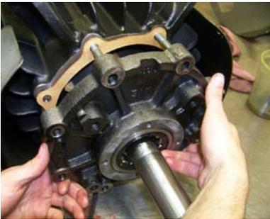
9. Install one (1) new endplate gasket between the housing and the endplate, **do not use any gasket sealer.**
