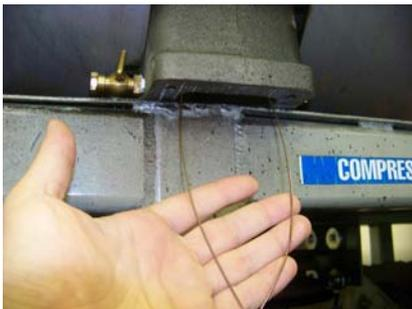
Divert the pull wire into the housing cavity and out through the intake port.
