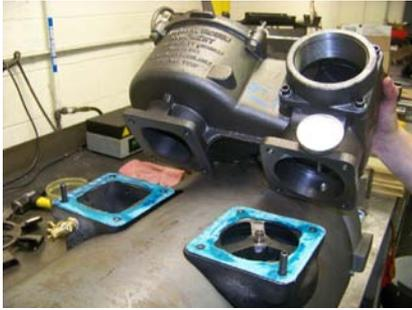
28. Install two (2) four-way gaskets to the housing interface.
