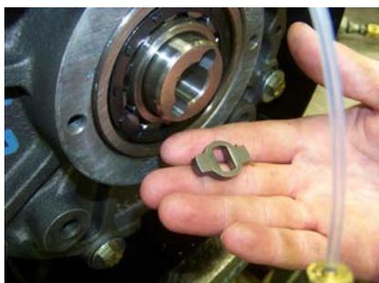
At this point you should be able to turn the rotor by hand.
