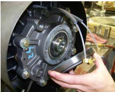
3. Remove the four (4) bolts that hold the rear bearing cover to the rear endplate and remove the rear bearing cover.
