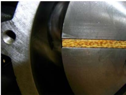
We highly recommend replacing vanes in sets. Apply a liberal amount of lubricant to the vanes before installing in the rotor slots.
