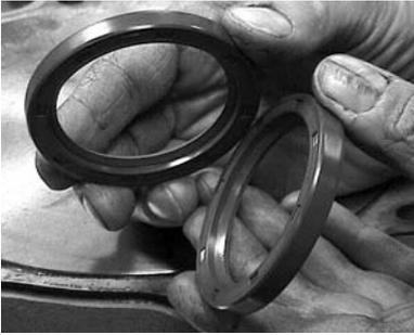
20. Remove the seals from the endplates. Inspect for damage, the seals should be soft and pliable.
