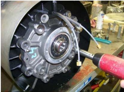
6. Remove the top two (2) bolts that hold the rear endplate to the pump housing and replace with two (2) 3/8-16 threaded dowels. Once in place, remove the lower six (6) 3/8 hex bolts.
