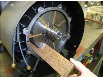
7. Remove the rear end-plate with a gentle "wiggle", clean gasket surface and remove the vanes for inspection.
