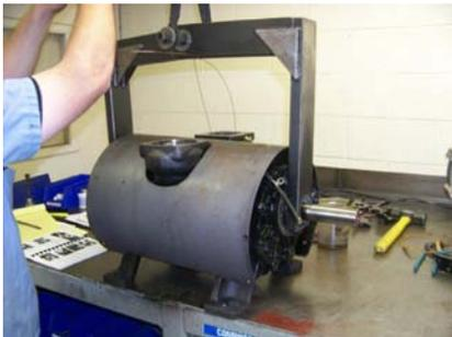
Tighten the endplate bolts to 35-40 ft-lbs of torque.
