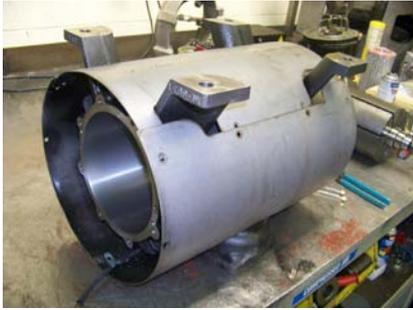
12. Remove the four-way assembly, gaskets, and check valve assembly. Carefully turn the housing upside down so that the pump feet are facing the ceiling.
