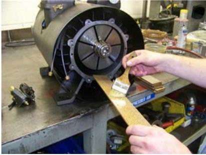
18. Inspect the original vanes for any delamination, chipping or other damage.
