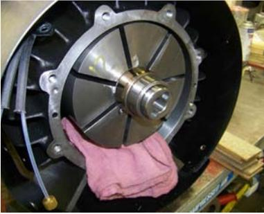
8. Place a cushion beneath the rotor to prevent damage when the front endplate is unbolted (cardboard, rag, etc.).
