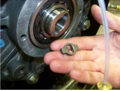
4. Remove the oil pump drive key from the end of the rotor.
