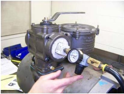
29. We highly recommend pressure testing your pump for leaks before putting it to work. We test our pumps at 20 psi of pressure.
