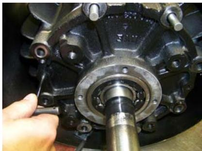
10. Insert the two (2) “T-handle” pins provided in your rebuild kit through the endplate and into the locator holes at 3 and 6 O’clock positions on the housing.
