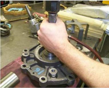
21. Lubricate the roller bearing pilot in the endplate. Using a bearing driver, seat the roller bearing into the endplate.
