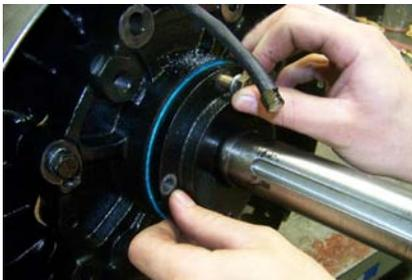
25. Reinstall the bearing cover gaskets, lubricate along the rotor bearing cover interface, reinstall the bearing covers (with wave washers installed)
