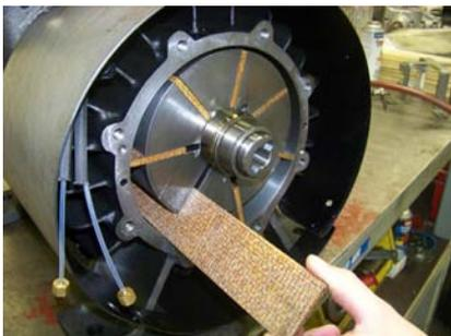
7. Remove the rear endplate, gasket, and vanes.
