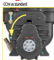
Version HM 125.7 cc/rev - Pmax 175 bar In G 1/2" - Out G 1/2"
