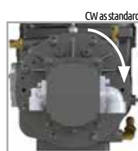
Version H Group 4 86,56 cc/rev - Pmax 280 bar - In G 1"1/4 - Out G 1" 1/2
