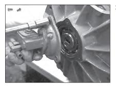
2. Remove the 3 6x20mm screws attaching the oil pump assembly to the vacuum pump.
