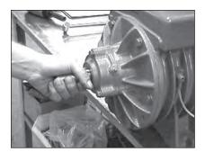
22. Lubricate and reinstall the front outboard bearing and bearing cover.
