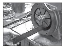
Coat the housing and vanes with oil and install the vanes in the rotor. The vanes should slide freely in the vane slot.
