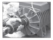
12. Lubricate seal sleeve and install the endplate on the end of the rotor and carefully drive the endplate on the rotor.
