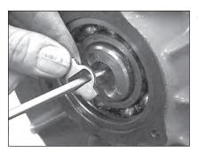
3. Remove the oil pump drive key from the end of the rotor.
