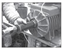
Tighten endplate bolts to 35-40 ft lb of torque.
