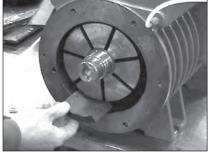
2. Place a cushion under the rotor to prevent damage when the front endplate is unbolted.
