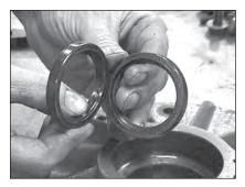
Locate the replacement seals and install them in the endplates with the seals positioned back to back.
