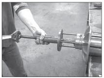
Remove the front endplate, 4. front bearing and bearing cover from the rotor with a puller or hydraulic press.
