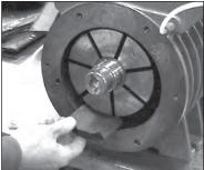
13. Slide rotor-endplate assembly into the pump housing.
