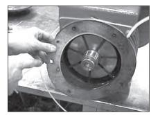
Note the number of gaskets on the endplate. You must use the same number of gaskets during reassembly.
