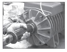
16. Locate the proper number of gaskets and install them on the rear endplate.
