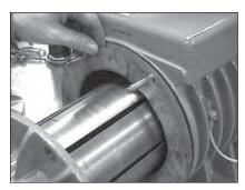
Locate two pieces of threaded rod 3/8-18 thd. to use as guides and screw them into the two top holes in the housing.
