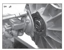
16. Reinstall the oil pump drive key and oil pump mount assembly to the pump.
