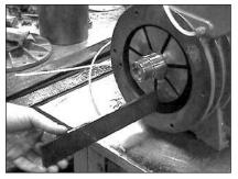
15. Coat vanes with oil and install the vanes in the rotor. The vanes should slide freely in the vane slots.
