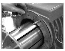
10. Locate two pieces of threaded rod 3/8-18 thd. to use as guides and screw them into the two top holes in the housing.
