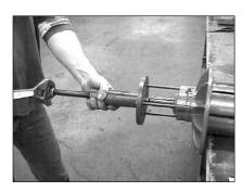
Remove the front endplate, front bearing and bearing cover from the rotor with a puller or hydraulic press.
