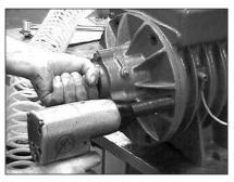
3. Remove the six bolts attaching the endplate to the housing.
