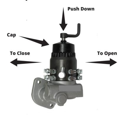
When the pump has been inoperative for 48 hours or longer, push down and hold down the spring loaded crank on the oil pump, while rotating the handle about 20-30 turns either way, or until oil drops can be seen dripping in oil flow valve.
