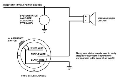
THE RELAY IS NEEDED IF THE HORN OR LIGHT DRAWS MORE THAN 1 AMP
