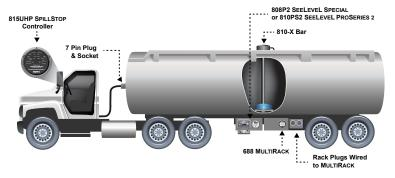
The SPILLSTOP controller works in conjunction with alarm signals sent by the 808P2 or 810PS2 level gauges, PTO position sensors and hose pressure sensors.
