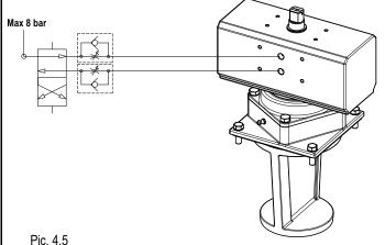
We recommend adjusting the two flow regulators in order for rotation to occur without knocks and with a switching time of at least one second.
