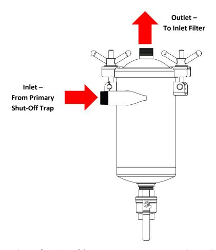
Whatever the configuration of the vacuum system on your truck or trailer, all components and plumbing must be of adequate size or the system will not operate correctly.
