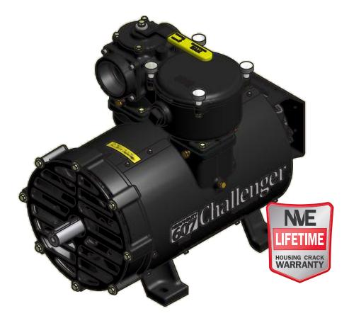
\*The maximum allowable operating vacuum will vary depending on R.P.M., ambient temperature, altitude and time running. The basic principle to keep in mind is - faster R.P.M., higher air temperature and longer run time all equal more heat in pump. When installing an NVE 607 pump we recommend a normal R.P.M. of 1250. Other speeds are ok as long as exhaust gas temperatures read on the supplied thermometer do not exceed 380 degrees F.
