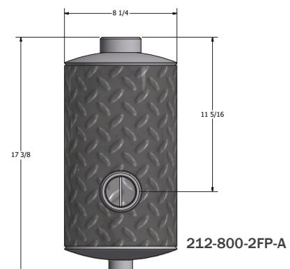
**8" and 12" Oil Catch Mufflers - Vertical Orientation**
