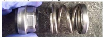
5) Start the seal on the shaft & press it on with a 7/8" socket.
