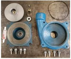
2) Rub a dab of grease on the wall were the seal seats. Grab the seal & press it into the adapter (press the seal in with the cardboard piece provided or use new clean gloves).
