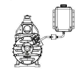
The oil reservoir tank must be mounted higher than the oil feed connection on the pump to ensure that oil will be fed by gravity to the oil pump.
