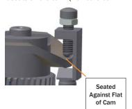
5. Back the screw off the desired amount of turns (CCW) - 5 turns if running at 900 RPM
